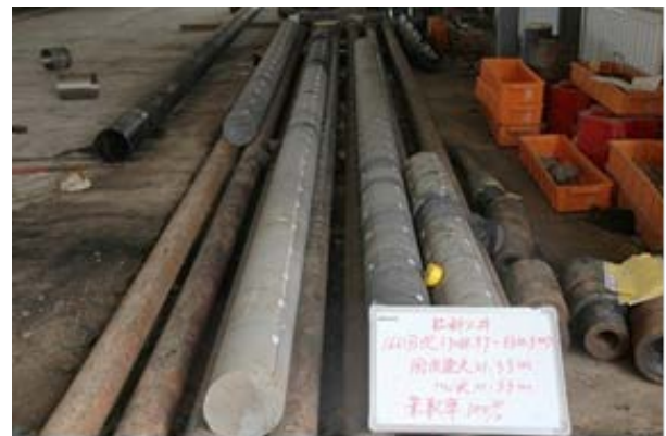
New record in drilling: 21.33 m core with 214 mm diameter
