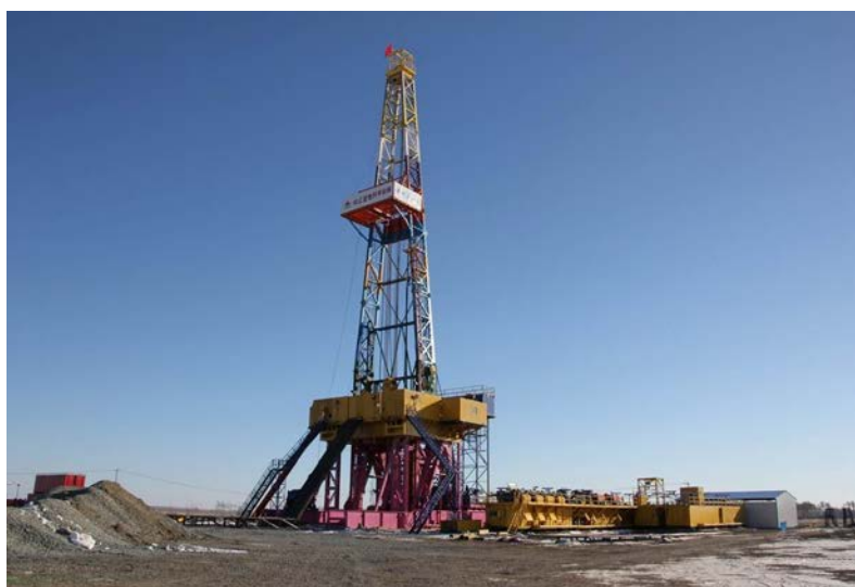
Crust-I, the new Chinese drill rig with 10 km depth capacity
