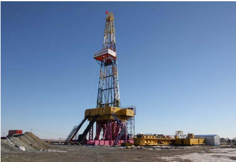
Crust-I, the new Chinese drill rig with 10 km depth capacity. Photo source: Qingtian Lu
