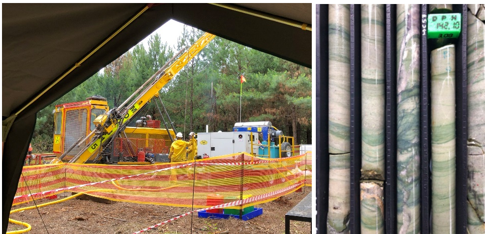
Drill Hole 4-1 and core samples taken from it in the BASE drilling campaign.
