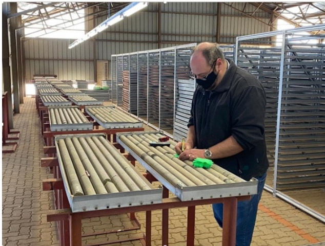
Marking and logging drill cores from the Bushveld Complex Main Zone. Photo: J. Magson, University of the Free State, South Africa.
