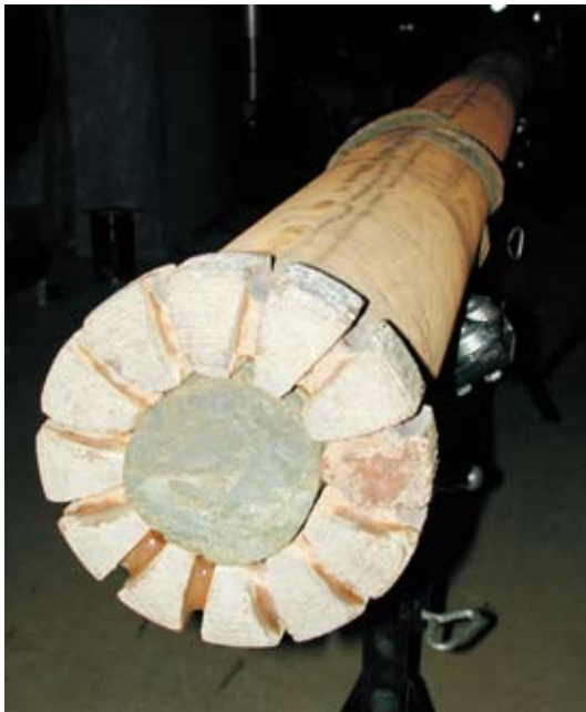
Figure 7. Core bit with core securely held in catcher.
