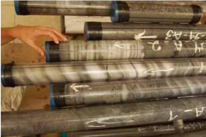
**Figure 2.** Drill cores in liners recovered at depth around 300 m below lake floor. From top to bottom the cores show change from gravel (top core) to marls interlaced with fine-grained salt layers (middle cores). This suggests that at that time the shore was very close to the drilling site, and the wavy salt patterns were interpreted as a result of salt flow.
