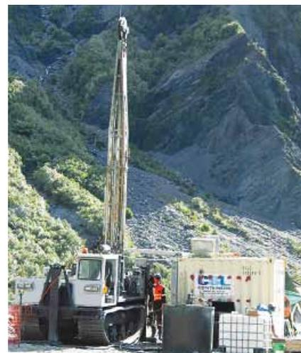
but the fault has now been resealed in both boreholes with a bentonite-cement grout. All aspects of the project were successful. High-quality cores and a comprehensive suite of wireline logs were collected from both boreholes. DFDP-1A has a seismometer installed at a depth of 83 m, just below steelcasing. DFDP-1B has a seismometer, 4 piezometers, and 24 tempera-
