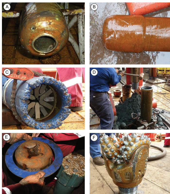
Figure 6. Photographs of some drilling, fishing, and milling tools illustrating the multiple operations achieved during IODP Expedition 335. [A] & [B] Remains of the Ultrera C9 RCB coring bit used during Run 9. The bit was probably used for ~10 h after it disintegrated, which resulted in this spectacularly abraded and sculptured bit ("Stumpy"), something never seen before by the drillers. [C] Bottom of the Bowen Reverse Circulation Junk Basket (RCJB), showing its hard-facing structure and the junk catcher spring fingers inside. This tool recovered a series of large-scale cobbles (up to 5 kg) of granoblastic basalt. [D] A series of RCJB runs returned a bottom hole assembly packed by fine-grained cuttings. This contributed efficiently to cleaning Hole 1256D. [E] Heavily worn and under-gauge 9-inch flat-bottomed milling tool. This tool worked at the bottom of the hole for 12 h; its final state indicates the very abrasive nature of metal debris and/or rocks at the bottom of the hole and an under-gauge lowermost portion (tens of centimeters) of the hole. Note for comparison the hard-facing structure of the next milling tool on the right side of the picture. [F] 9-inch Smith FH3VPS tricone bit used for Run 16. This armored bit was efficient to ream and clean the under-gauge bottom of the hole.
