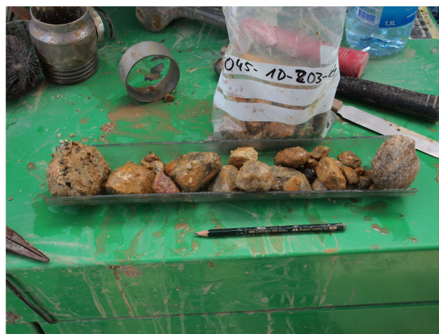
Figure 8. Rounded gravel and pebbles in core catcher material (DEEP site, hole 1D at 569 m b.l.f.) indicate fluvial transportation.
