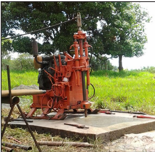
Figure 4. The drilling rig used to retrieve core material for this study was mainly oriented perpendicular to the strata truncated.
