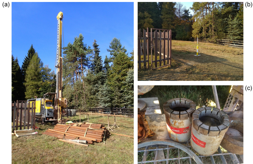
Figure 3. The Eger Rift drilling setup, showing (a) the drilling rig with drilling rods at the S3 site, (b) the wellhead after the termination of work at the S3 site and (c) an example of a diamond drill head designed for drilling in hard rocks.
