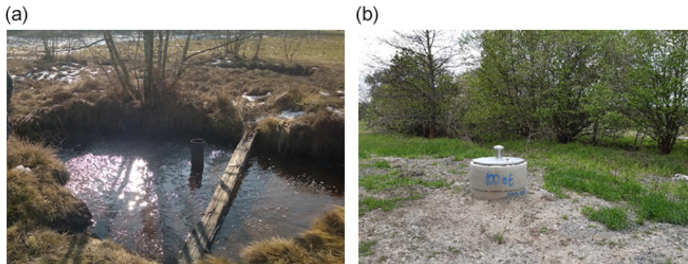
Figure 4. Panel (a) shows the Hartoušov mofette field, and panel (b) presents the F3 borehole in Hartoušov after the completion of drilling works, with the concrete head casing secured by a lock.
