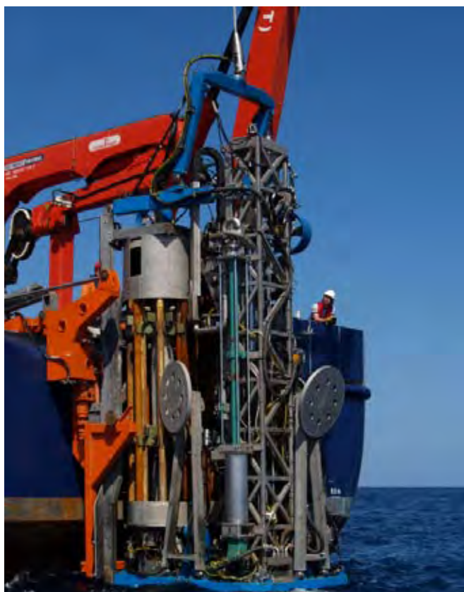
Figure 5. Launch of the sea floor drill rig MeBo from the Maria S. Merian .
