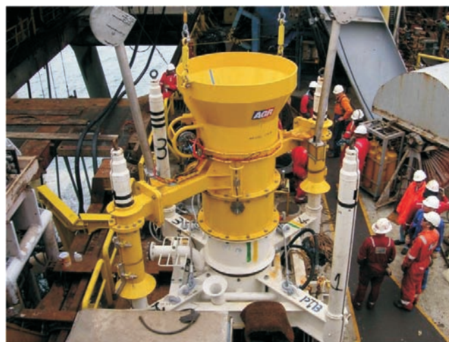
Figure 4. The AGR riserless mud recovery subsea equipment consists of a mud suction module (see above) and seafloor mud pumps. The mud is collected in the mud suction module and returned to the drillship via the seafloor mud pumps (image: courtesy of John Thorogood).
