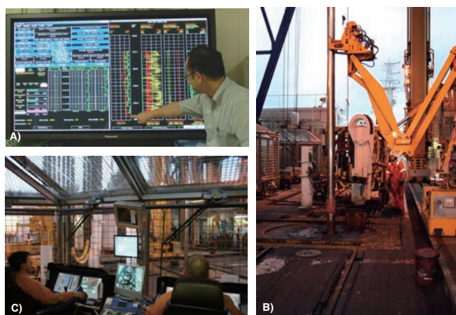
Figure 3. LWD drilling operations during Expedition 314. [A] Real time monitoring in the lab area; [B] LWD toolstring on the rig floor; [C] Driller's house operations.
