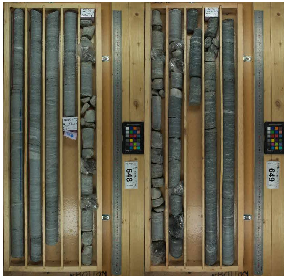
Fig. 4.5.4: Core boxes 648 and 649 from COSC-1. The core boxes are used in portrait format (=upper left corner = Top, lower right corner = Bottom. Top and bottom of core runs are marked with labelled foam blocks. Each box was photographed with the cm/ft ruler and a standard colour chart.
