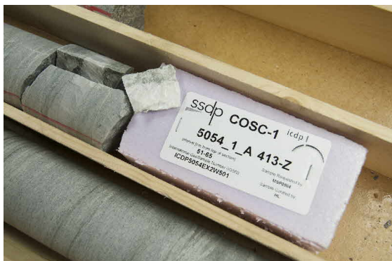
Fig. 4.5.5: Sample location filled with a labelled foam block showing the sample number and IGSN (lower left: ICDP5045EX2W501)
