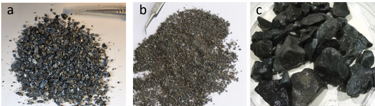
Fig. 4.5.17(a) cuttings of mica schist taken during the DFDP drilling project in New Zealand, (b), cuttings of a mixture of sand/silt and claystone taken from the SAFOD drilling project in USA, (c) cuttings of silty claystone, siltstone and sandstone taken during the NanTroSEIZE drilling project in Japan (cm scale).
