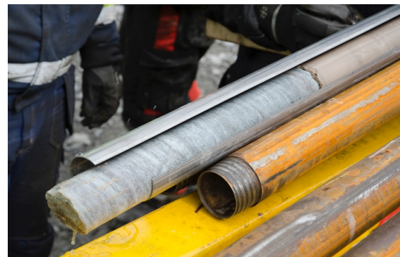
Fig. 4.5.1: First COSC drill core (gneiss below cement) in opened inner tube of a triple tube core barrel assembly. Clearly visible is the split aluminium liner protecting core from external forces, the second tube, and the drill string tube, hence 'triple tube'.
