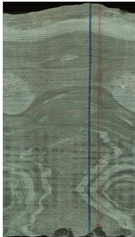
Fig. 4.5.3: Whole round optical core scan of gneiss core section showing double reference line in upright position with red line on the right
