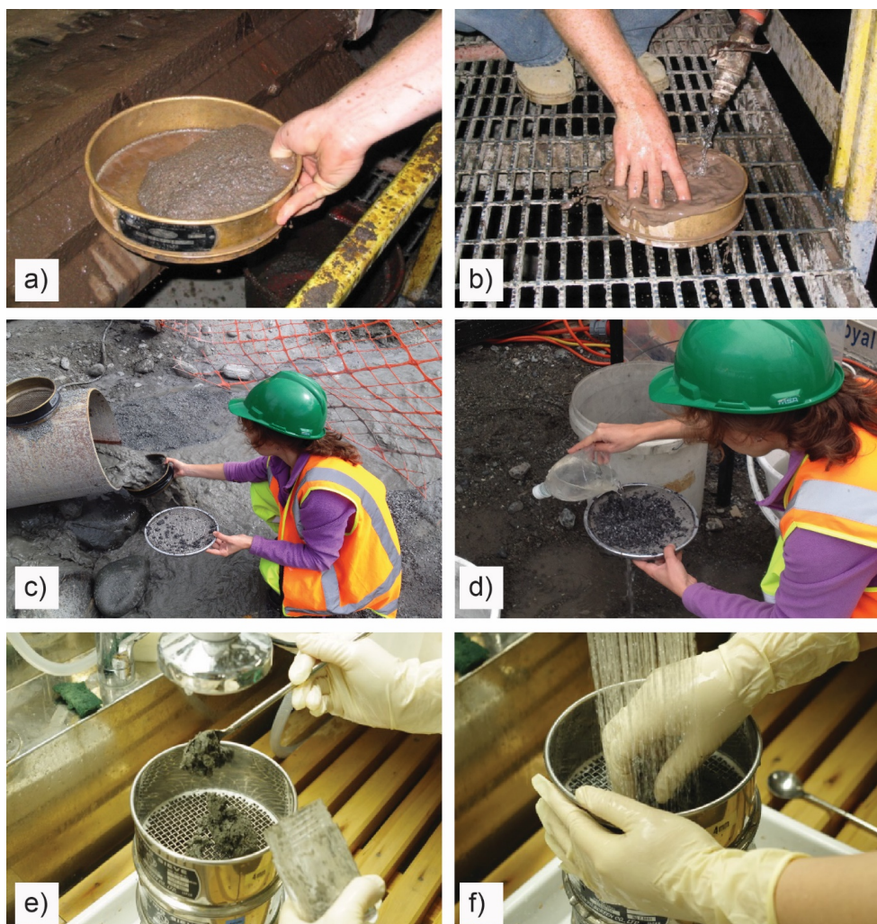
Fig. 4.5.18: a) and b) cuttings were separated from the liquids at the shale shaker and later washed with tab water (SAFOD); c) and d) cuttings were collected directly at the drilling mud outlet and rinsed later with tab water (DFDP); e) and f) chip size separation (< 2mm, 1-4 mm, > 4mm) and rinsing of cuttings after collection at the shale shaker (NanTroSEIZE).
