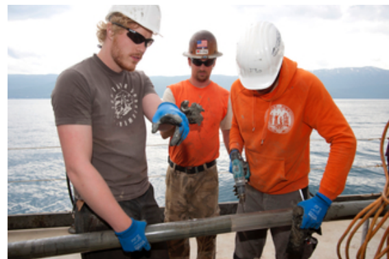
Fig. 4.5.7: Drill core handling on the barge. Small holes were drilled into plastic liners to prevent excessive core expansion from high gas pressure in the liner (Photo: N. Leicher).
