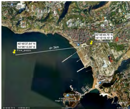
Fig. 4.2.9: Horizontal well trajectory for the Campi Flegrei deep drilling project in Italy
