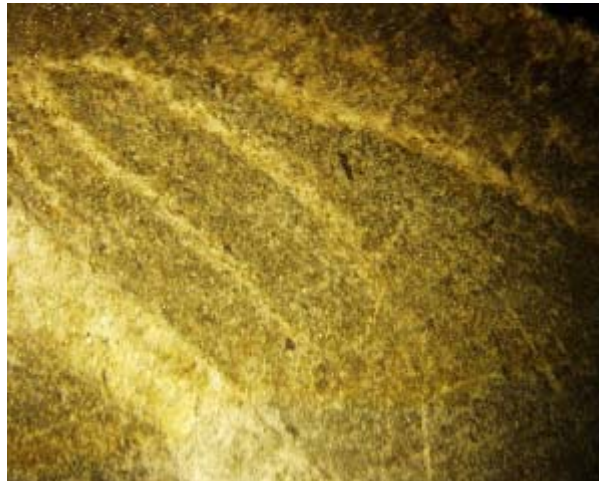
Fig. 29 : Microscopic observation of the shear zone of sample S27
