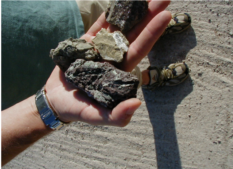
Figure 7 : Samples of rock pieces eroded from the fault gouge because of the high production flow rate.
