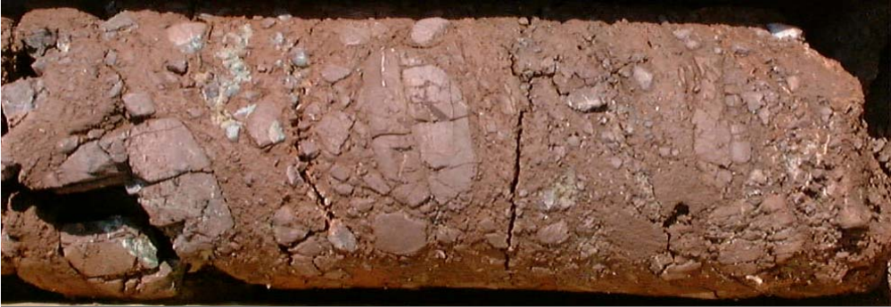
Fig. 9. 100mm diameter core of radiolarite-derived fault gouge (760m AIG10)
