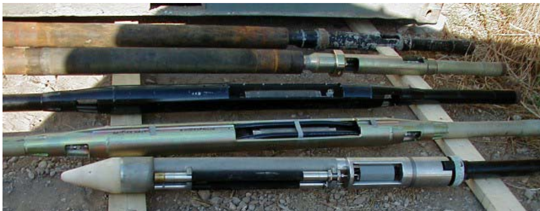
Figure 3 : In the foreground : the seismometer cell with its two packers for downhole coupling; in the background : the two high pressure packers
