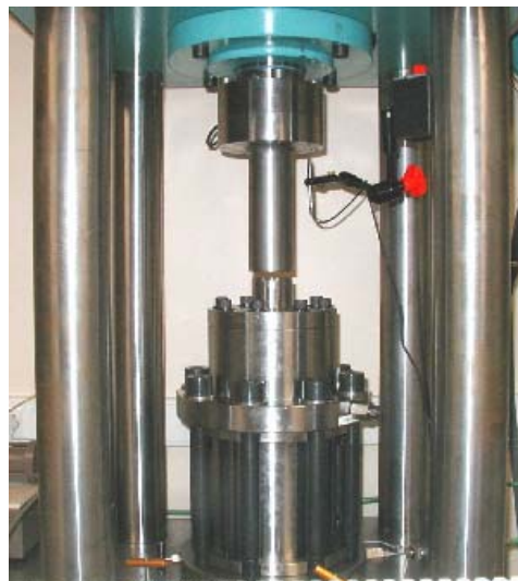
Fig. 18 : Triaxial cell and loading frame
