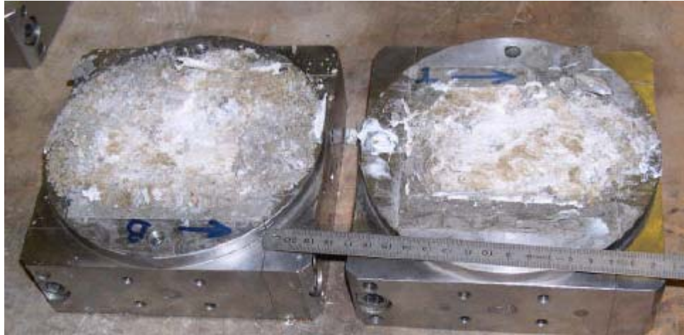
Fig. 16 : The contact zone between the limestone and the breccia tested in direct shear
