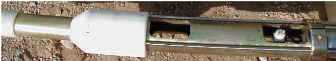
Figure 4 : Close up view showing the electrodes for water conductivity
