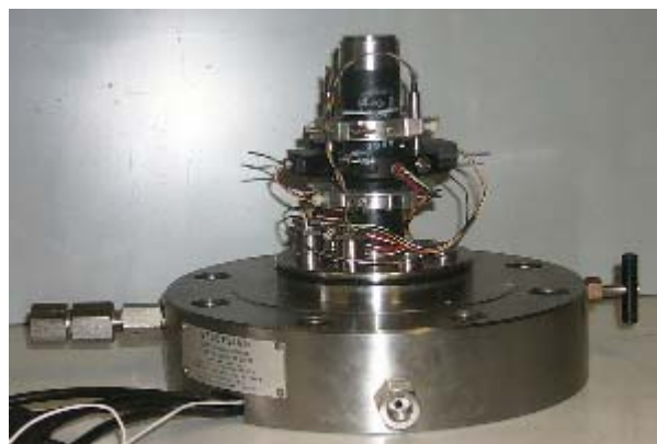
Fig. 20: Instrumentation of the sample inside the cell
