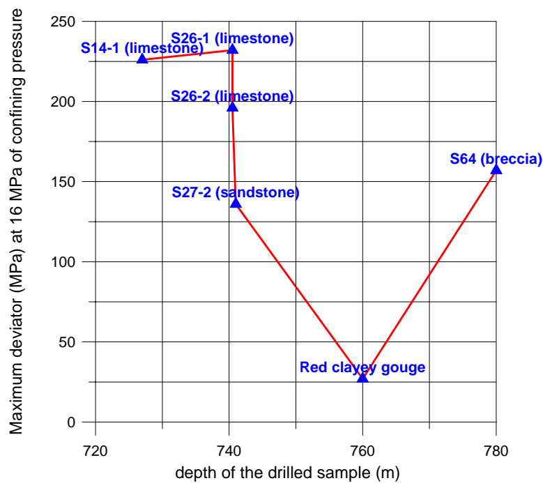
Fig. 24: Maximum deviator profile at 16 MPa of confinement
