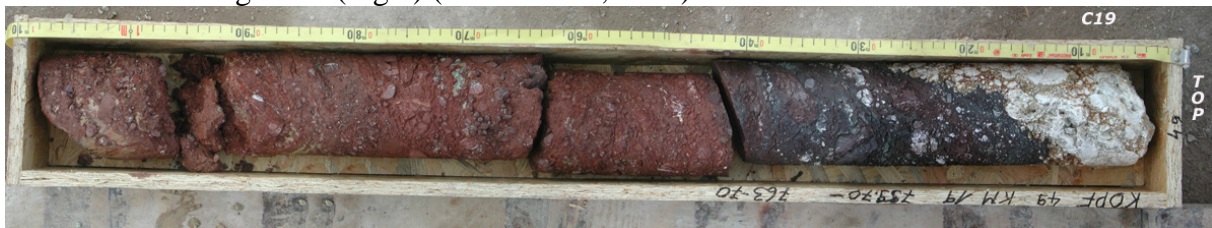
Fig.1. Box 49 containing the core at depth 759.70m, characterised as “Aigion fault” core (Moretti et al, 2003)
